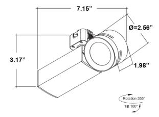
Sleek and compact, this 12.5 W / 700 Lumen LED track light has an integrated driver; is adjustable with 355° rotation, 100° tilt; and, eco-friendly with no heat, UV, or IR radiation, so will not degrade fabrics or artwork. It is an excellent choice to highlight artwork or displays. Suitable for residential, commercial, or retail applications.
