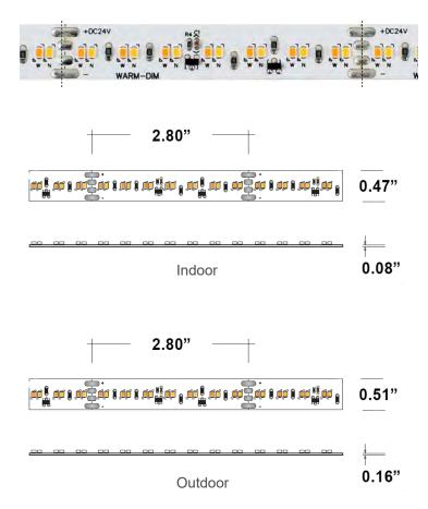
TBD.SWD3.64(W) is an auto warm-dim indoor/outdoor strip. Utilizing a standard dimmer, will shift color temperature from 3000K to 1800K. Great new smart chip technology provides a very cost effective option for warm-dim.
