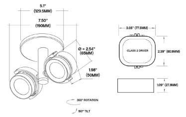
Sleek and compact, this 20W / 1200 Lumen Dual LED monopoint is adjustable with 355° rotation, 150° tilt; and, eco-friendly with no heat, UV, or IR radiation, so will not degrade fabrics or artwork. It is an excellent choice where extra adjustability is needed. Suitable for residential, commercial, or retail applications.
